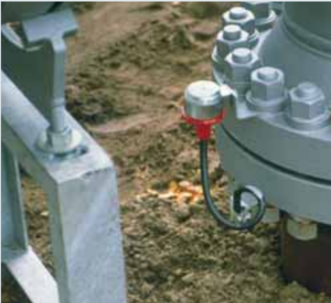
ATEX-certified isolating spark gap for lightning equipotential bonding according to IEC 62305, approved device with flexible conductor connection
